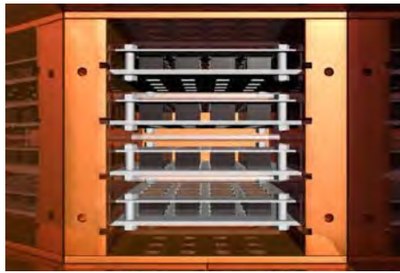
Figure 6. Schematic layout of the COBRA 64 array in the form of a 4 \times 4 \times 4 configuration. Each layer contains 16 CdZnTe semiconductor detectors.
