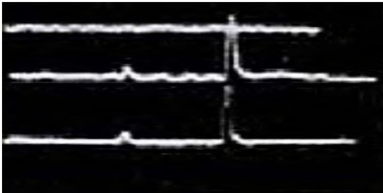
Figure 4. Example of inverse beta decay signal from Savannah River experiment recorded on an oscilloscope (Reines et al. 1960). Copyright (1960) American Physical Society. The three traces show signals from tanks I, II, and III (see Figure 3).
